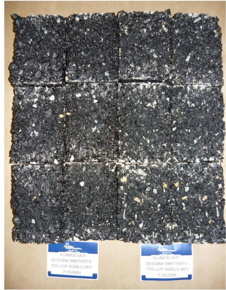
ILLDOT Design No. 39BIT9381V 0.75% AD-here LOF 6500 LS
